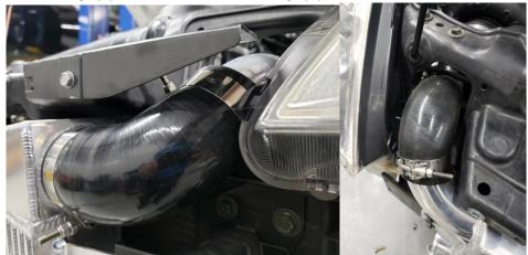
141. Install the single reducer coupler onto the bottom endcap of the intercooler and the one 45 degree 2.5" coupler onto the turbo. Once you have installed these couplers, proceed to installing the charge pipe.
