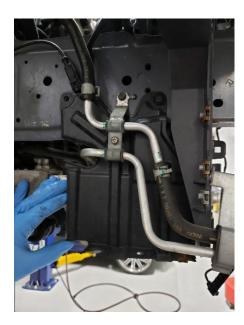
15. Using a 10 mm socket remove the power steering line bracket and unhook the power steering cooler lines from the radiator support.
