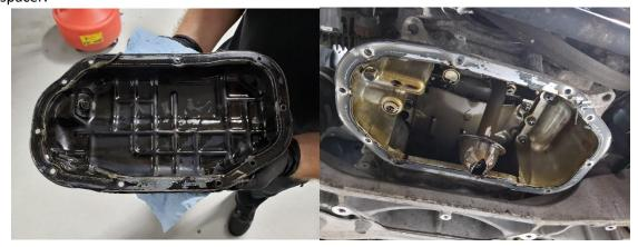
109. Remove the two (12 mm) bolts that hold the oil pick up as you will be adding a spacer to allow the pick-up tube to work properly with the new spacer.
