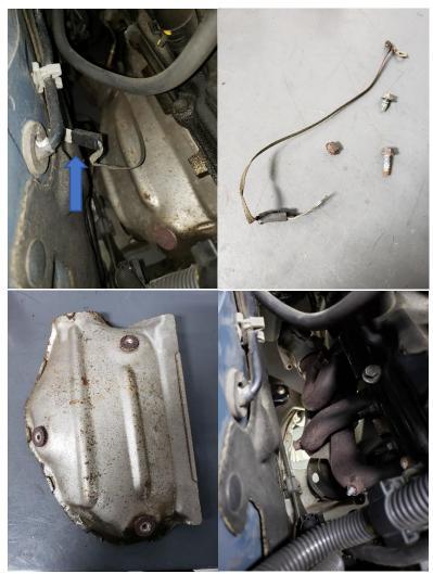
19. Remove the lower heat shield located on the manifold which can be seen below.
