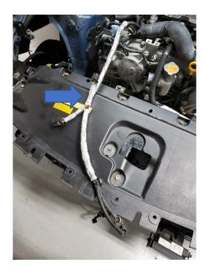
39. Route the alternator wire along the alternator and the starter wire across the top of the timing cover.
