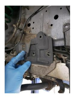
14. Remove the large plastic cover behind the power steering lines as seen below.
