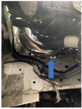
124. Now you will need to install the passenger side charge pipe prior to installing the top portion of the downpipe, as there is very little clearance once the passenger side charge pipe is installed.
