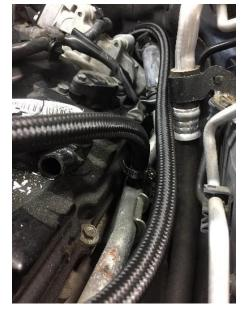
135. Route the other line with the 45 degree fitting to the rear of the engine and secure it onto the hard line as seen below.
