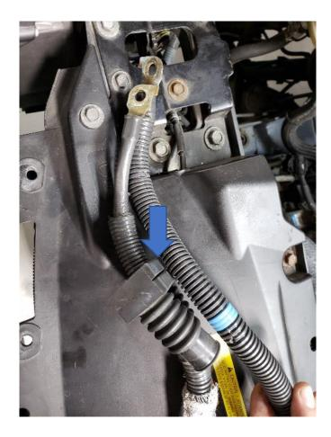
34. Slide the starter cable to the right along the engine harness bracket on the front of the motor as seen below and zip tie the excess cable to the chassis harness located on the driver's side.
