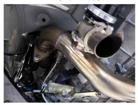
122. Install the up pipe onto the crossover section and be sure to use the 3" v-band that has been provided. Note to orient the clamp as shown in the picture below.
