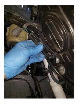
10. Remove the line connected to the windshield washer reservoir and allow the fluid to drain, while the fluid is draining remove the driver's side front fender liner.
