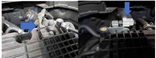
55. Remove the two bolts that hold the stock evap lines and vacuum lines as seen below on the back of the throttle bodies.
