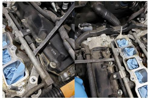
65. Slowly pull out the fuel rails as you will need to disconnect the rear connector to the injector harness as seen below.
