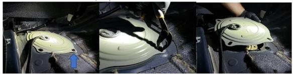
78. Pick up the fuel pump cover and locate the main fuel pump connector and remove the connector.
