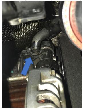
51. Route the rubber line next to the AN hard line to the bottom port of the power steering oil cooler, be sure to add a section of black heat sleeve as you get closer to the power steering rack. Also ensure to rout the harness as routed in the picture below.
