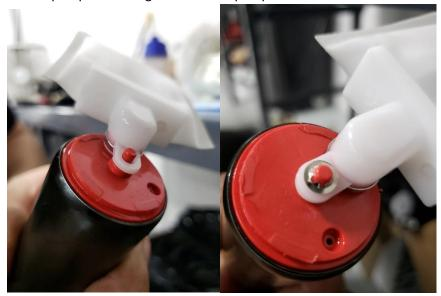
93. Remove the plastic cover on the fuel pump inlet and install the black rubber grommet, once these items have been installed onto the fuel pump, install the fuel pump into the stock fuel pump housing.
