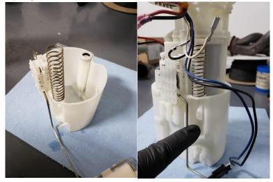
98. With the fuel pump housing now back together, reinstall the fuel pump level harness and position the harnesses out of the way of being damaged.
