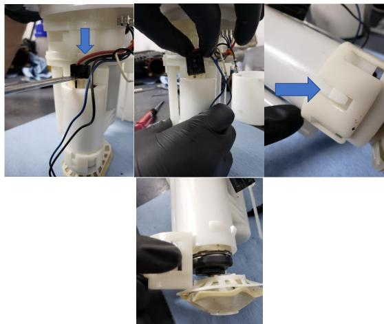
89. Press down on the top of the fuel pump as you pull the fuel pump thru the housing.
