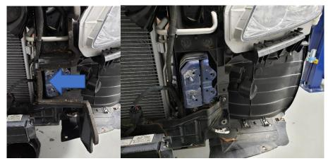
5. Remove the top bolt and plastic clips that hold plastic intake duct into place on both sides as seen below. Passenger side will have harness clip that will need to be removed prior to removing plastic intakes.
