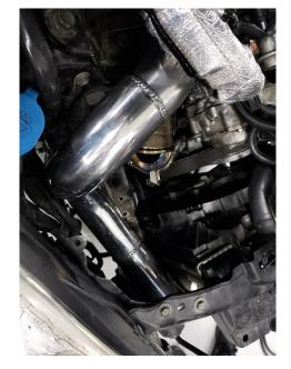
125. Prior to installing the turbo ensure that the compressor side of the turbo is clocked towards the radiator fan assembly. Also install the top portion of the downpipe as seen in the picture below.
