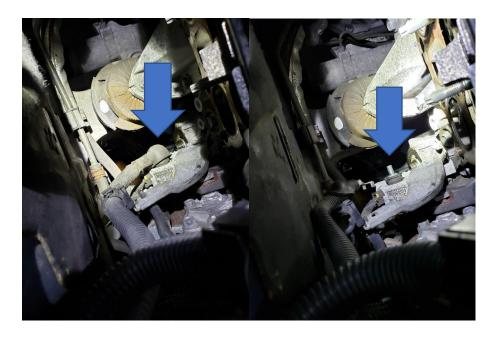
26. You will need to modify the plastic housing that sits in the alternator assembly by sanding down the rounded corners on the plastic housing as seen below. You will need to test fit the plastic housing after sanding down the corners to ensure that it will fully turn in the alternator once installed as seen below.
