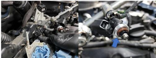
71. With the fuel injectors and fuel rail installed, proceed to installing the fuel hard line as seen below using the two 10mm and one 12mm bolt. Please lubricate the oring on the one end of the hard line and check that the oring is not torn.
