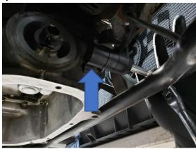
111. Install the straight gold adaptor fitting into the location of the stock OEM oil pressure sensor, slowly tighten the gold fitting into the upper oil pan until it is snug. Take caution to not over tighten this fitting as you will crack the upper oil pan. With the adaptor fitting installed, apply thread sealant to the three way fitting and install this fitting into the other fitting.
