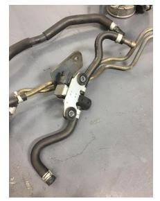
133. Install the black coolant lines that have been provided in the kit labeled HR\_SMCL1 & HR\_SMCL2. The coolant lines both have a 45 degree fitting, the longer line will need to go to the far left part of the turbo.
