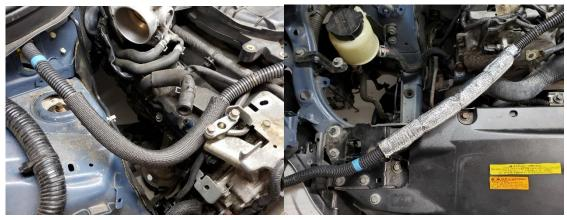
36. Locate the two sensor connectors on the lower passenger side of the engine and disconnect them at this time as seen below.
