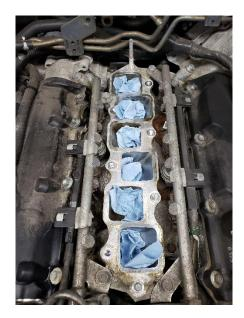
61. With the intake manifold removed, remove the clamp holding the coolant line to the throttle body on the driver's side as seen below.
