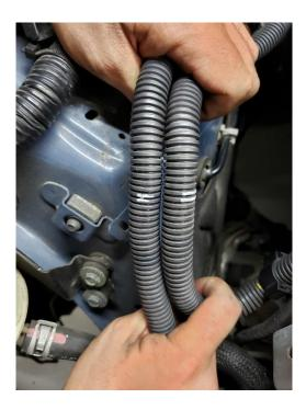
30. Locate the alternator wire and remove the black tape that is holding the alternator boot onto the heat shielding. Once the black alternator boot has been removed, you will need to install the black heat sleeve provided onto the OEM harness and heat shield.
