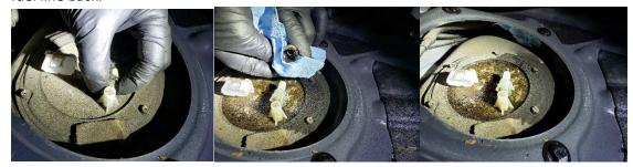
81. Locate the six 8mm bolts that hold the fuel pump bracket to the chassis and begin to remove them. Be careful to hold the fuel pump assembly down when removing the last bolt as the fuel pump assembly will want to push upwards.
