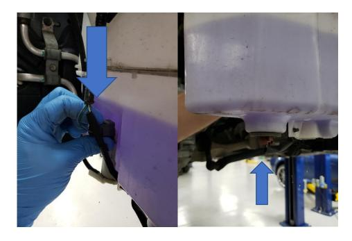
9. Using the zip ties provided, zip tie the windshield washer harness to the main headlight housing and away from the tire.
