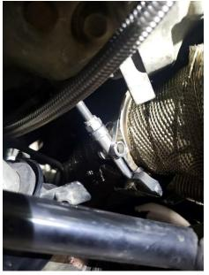
123. With the up pipe installed, you will now need to trim part of the frame to allow for the passenger side charge pipe to clear the turbo, which can be seen below.
