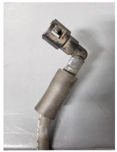
41. You will now wrap these two lines with the black heat sleeve, one will require a 21.5" section and the other will require a 16" section, which can be seen below.
