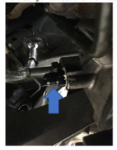
49. Route the high-pressure power steering line from the power steering rack adaptor fitting to the power steering pump adaptor fitting. When routing the line be sure to route the line above the hard line as pictured below and close to the engine as you make your way up to the power steering pump.
