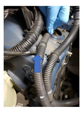
28. Once the clips have been removed, remove the zip tie in the larger of the two clips as it will be used again to hold the harnesses to the chassis.
