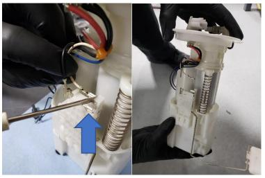
88. Disconnect the fuel pump main connector and the plastic housing underneath the fuel pump as shown below.
