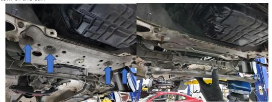
104. Unhook the tabs that hold the power steering harness and connector to the secondary OEM skid plate as shown below.
