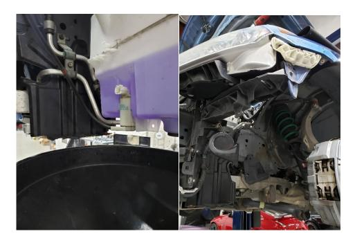
11. Once the fender liner has been removed, relocate the horn as shown below.
