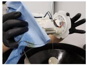
85. Apply pressure to the top of the fuel pump and lift on the lever as shown in the picture below to separate the fuel pump hosuing. Be careful not to completely remove the fuel pump out of the housing when removing the lever and it will move upwards.
