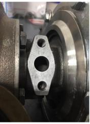
117. Install one end of the -8 AN oil drain line to the fitting and be sure that the fitting is tight.
