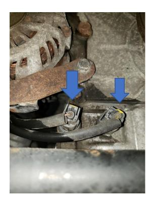
37. Move the smaller harness that has the two connectors up towards the front of the engine as you will now start to install the reflective heat protectant onto this harness.
