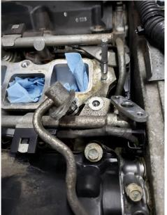
Note: When removing the hard line, be careful to not damage the black o ring
