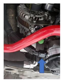
138. Install the upper intake manifold back onto the vehicle via the 6 bolts and two nuts.
