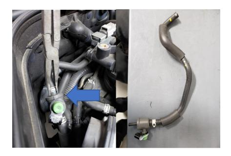
23. With the evap line removed, begin to remove the two (10 mm) bolts that hold the stock fuel pressure regulator on top of the engine and remove the fuel line.
