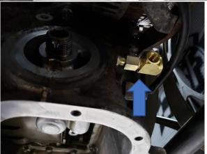
112. With both of the gold fittings installed, reinstall the OEM oil pressure sensor into the port that is closest to you and install the silver -4 oil feed fitting into the adjacent opening.
