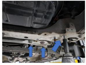
106. Remove nine of the ten (10 mm) bolts that hold the lower oil pan spacer to the engine, leaving the one bolt closest to the oil drain bolt so that the oil pan will not fall.
