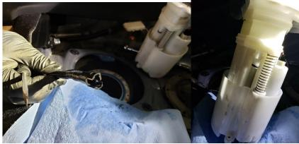
84. Remove the fuel pump assembly out of the vehicle and drain any excess fuel that may remain in the fuel pump assembly.
