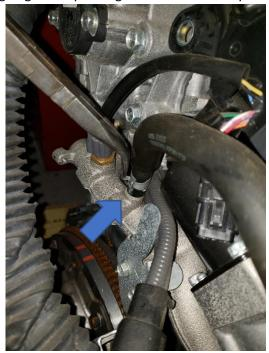
63. Remove the four (12 mm) bolts that hold the fuel injector rails along with the two (10 mm) bolts that hold the other end of the hard line for the OEM stock fuel pressure regulator.
