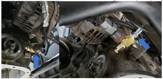
113. Locate the oil pickup tube spacer and install it along with the oil pick up tube as seen below.
