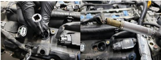
75. Install the new spark plugs and install the coils back into their original location.
