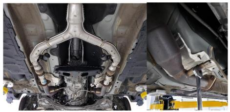
17. Remove the passenger side heat shield.
