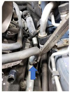
62. You will now move towards the rear of the engine and remove the coolant line that is mounted in the back of the engine going to the passenger side throttle body.
