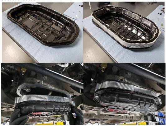
115. With the oil pan spacer installed, install the drain plug for the spacer along with the SOHO oil pan adaptor fitting.
