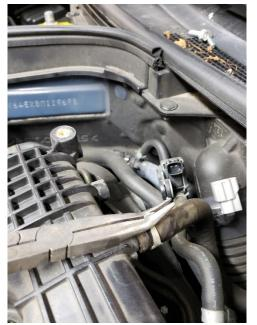
58. Remove the four bolts that hold the throttle bodies to the intake manifold (*H5 socket*)
