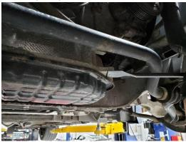
**Caution:** You will need to slowly work the screwdriver up and down to remove the oil pan spacer as the RTV that is holding the lower oil pan spacer has hardened over time.
