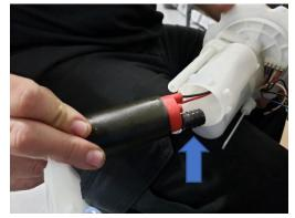
94. Install the plastic cover to the bottom of the fuel pump housing to cover up the fuel pump.
