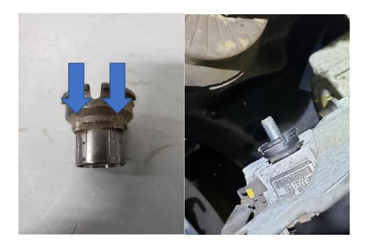
27. Remove the clips that hold the wiring harness to the chassis, be careful when removing the clips to not break them, as the clip on the left will be reused.
