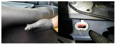
77. Once you have located the fuel pump, rotate the black tabs that hold the fuel pump cover clockwise and remove the fuel pump cover.
