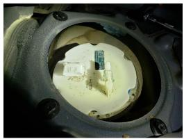
102. Install the metal housing and the 6 (8mm) bolts on top of the fuel pump housing, followed by attaching the main fuel line and connecting the main fuel pump connector. With everything attached, reinstall the metal cover over the fuel pump assembly.
