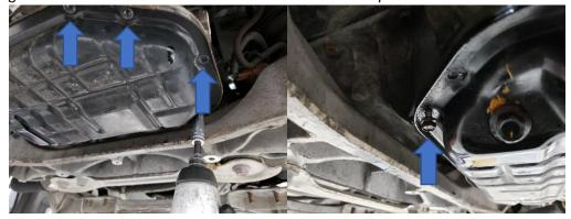
107. With the bolts removed from the lower oil pan spacer, use a flat head screwdriver and slowly begin to the remove the oil pan spacer as seen below.
