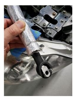
33. Remove the starter cable from the dual rubber grommet that is holding the alternator wire as pictured below.
