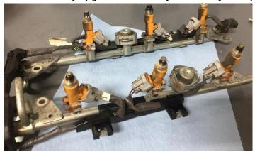
68. Remove the clip that is located on the bottom of the stock fuel injectors as seen below, gently apply pressure onto the fuel injector to remove them.
