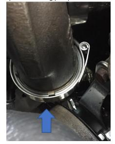
127. Install the turbo downpipe clamp onto the downpipe to secure it to the turbo as seen below.
