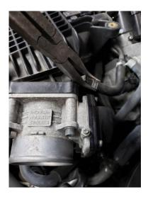
57. Remove the clamp holding the brake booster line found on the back of the manifold
