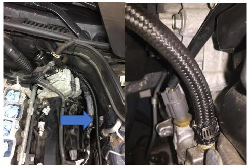
136. With both of the coolant lines run and installed, locate the oil feed line (HR\_SMFL) and install the 90 degree end onto the top of the turbo via the -4 AN fitting and the other end to the gold tee. Route the line down near the passenger side frame horn taking care not to have the line rub against anything that will get hot.
