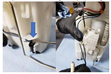
87. Remove the two wire connectors for the fuel level sensor as shown below and separate the fuel pump assembly.
