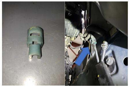
\*Be aware that fuel is pressurized and to have a towel over or near the line as you are removing the line\*
