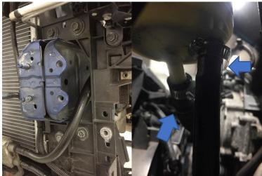
48. You will need to remove the OEM power steering lines that come off the power steering rack and install the power steering rack adaptor fitting.
