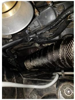
126. Install the v-band flange onto the stage one up pipe prior to installing the turbo onto the up pipe, as seen below. When installing the turbo direct the oil drain line down and close to the frame horn and away from the power steering pump.
