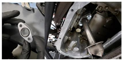
114. Using RTV, apply a film on the outer edge of the lower oil pan and install the oil pan spacer onto the lower oil pan. Repeat this process with the oil pan spacer and install it onto the vehicle as seen below.
