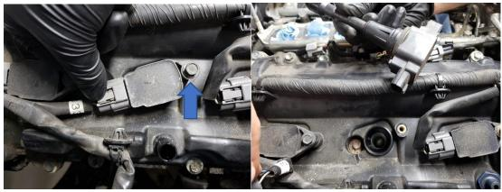
74. Remove the ignition coil and use a 12 point thin wall 14mm spark plug socket to remove the spark plugs.
