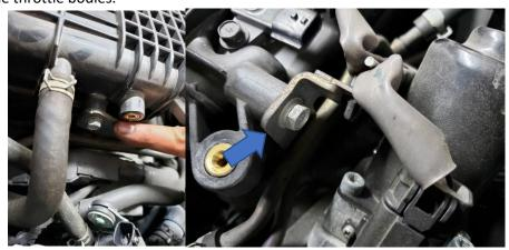
56. Disconnect the two vacuum lines to the manifold that are located on the back of the throttle bodies.
