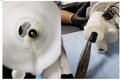
91. Locate the new fuel pump and proceed to sand down the four tabs on the bottom of the fuel pump to make the fuel pump flush.
