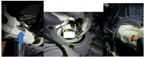
101. With the fuel pump installed into the fuel tank, make sure the orientation of the main fuel line on top of the fuel pump housing and the main fuel connector are oriented 180 degrees away from each other.
