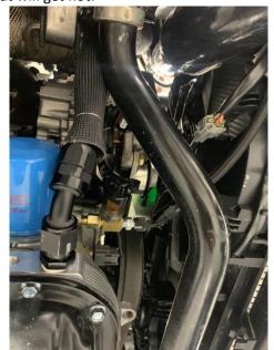
137. Install the oil drain line onto the black AN fitting on the oil pan spacer as seen below.
