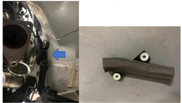
120. At this point, you will need to install the crossover section of the hot side turbo piping
