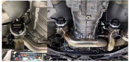
131. With the wastegate installed, install the fitting to the bottom port of the wastegate as seen below. You will need to run a vacuum hose to the back side of the manifold or to a boost controller if you have one, so make sure that you cut a long length to be able to reach where you plan on routing it.
