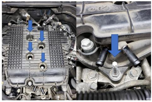
60. Remove the intake manifold and be sure to cover the lower intake manifold to prevent anything from falling into the engine.
