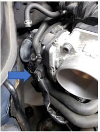
54. Disconnect the map sensor and evap pressure sensor connectors.
