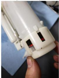
95. Since the new fuel pump does not have an OEM connector you will need to remove the current connector on the new fuel pump and on the OEM fuel pump housing. You will need to join the positive (red wire) from the fuel pump to the red wire of the OEM wiring harness and the negative (black wire) from the fuel pump to the black wire of the OEM wiring harness.
