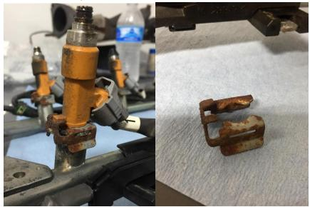
69. Prior to installing the new injectors onto the fuel rail along with the injector dynamic clips, be sure to lubricate the black oring on the injectors.
