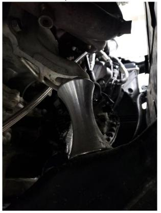
46. Remove the OEM power steering reservoir located on the passenger side and move it to the driver's side using the power steering relocation bracket.
