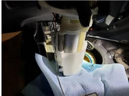
83. With the fuel pump removed out of the chassis, locate the black hose that is on the side of the fuel pump assembly. Remove this black hose by using a screwdriver to slightly press the tabs back and at the same time pulling the line off of the fuel pump assembly.
