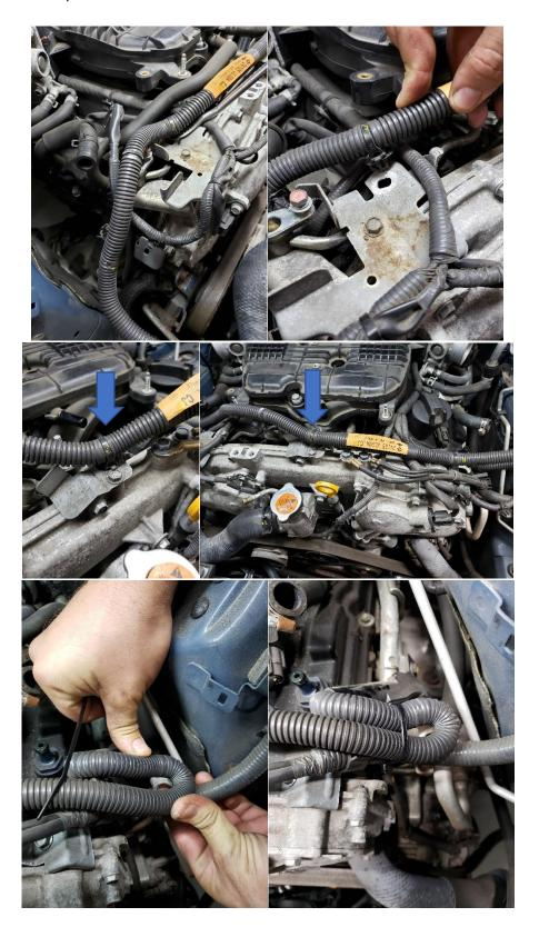
35. Install an 11.5" black heat sleeve section over the starter cable first, followed by a 12" reflective heat sleeve section over the black heat sleeve and safety wire or zip tie it secure.
