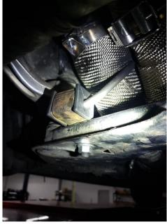
130. Install the Waste gate dump tube onto the wastegate, then install the wastegate onto the crossover pipe as seen below.
