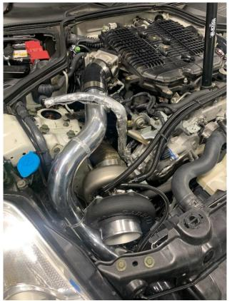
134. Zip tie both lines together up until you get to the front of the engine timing cover as seen below. Route one of the lines to the driver's side coolant hard line and secure using the hose clamps provided as seen below.
