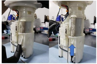
86. Disconnect the fuel temp sensor and harness along the fuel pump housing.
