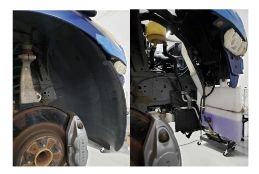
8. Unplug both harnesses on the windshield washer reservoir, one on the back and one on the bottom as seen in the picture below.
