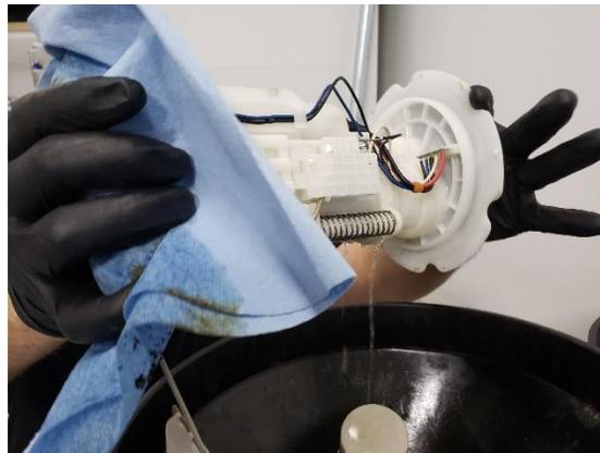
85. Apply pressure to the top of the fuel pump and lift on the lever as shown in the picture below to separate the fuel pump housing. Be careful not to completely remove the fuel pump out of the housing when removing the lever and it will move upwards.
