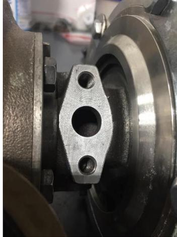
117. Install one end of the -8 AN oil drain line to the fitting and be sure that the fitting is tight.
