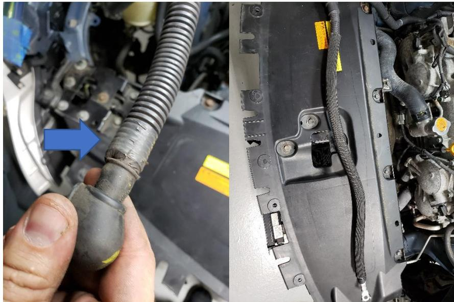
31. After the black heat sleeve has been installed onto the harness, you will need to install the reflective heat sleeve over the same harness and secure it with either safety wire or zip ties.
