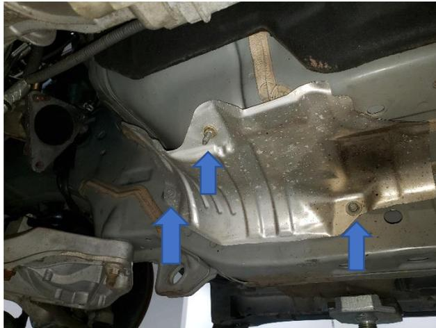
18. Remove the harness ground and manifold heat shield located on the passenger side of the vehicle.
