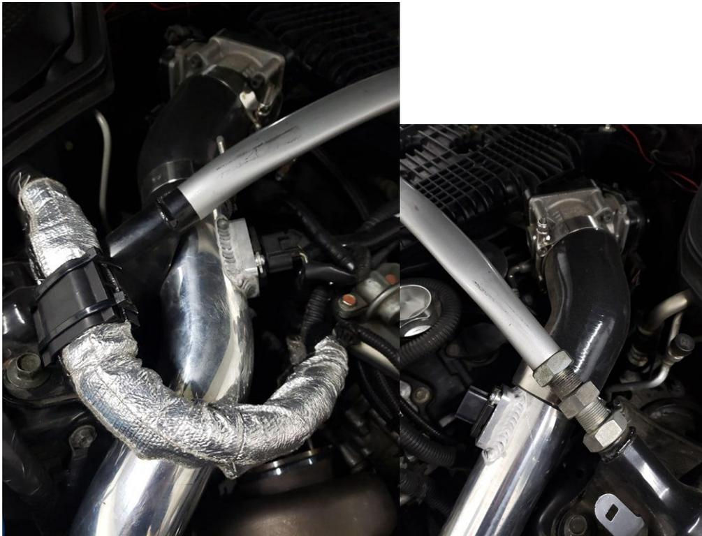
144. Install the fitting that comes with the blow off valve onto the blow off valve and then install them onto the flange and seen below.
