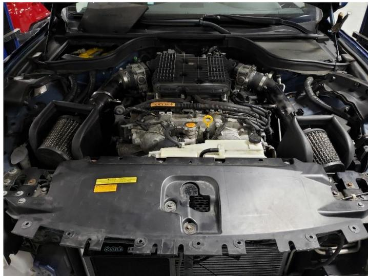
4. Remove front bumper and remove plastic trims along the frame horns.
