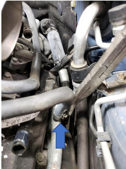
62. You will now move towards the rear of the engine and remove the coolant line that is mounted in the back of the engine going to the passenger side throttle body.
