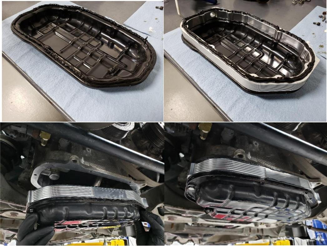
115. With the oil pan spacer installed, install the drain plug for the spacer along with the SOHO oil pan adaptor fitting.
