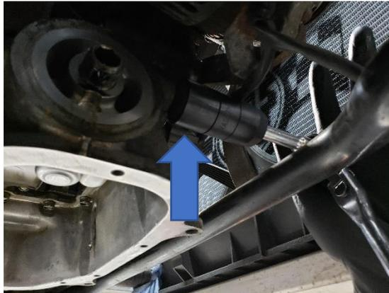
111. Install the straight gold adaptor fitting into the location of the stock OEM oil pressure sensor, slowly tighten the gold fitting into the upper oil pan until it is snug. Take caution to not over tighten this fitting as you will crack the upper oil pan. With the adaptor fitting installed, apply thread sealant to the three way fitting and install this fitting into the other fitting.
