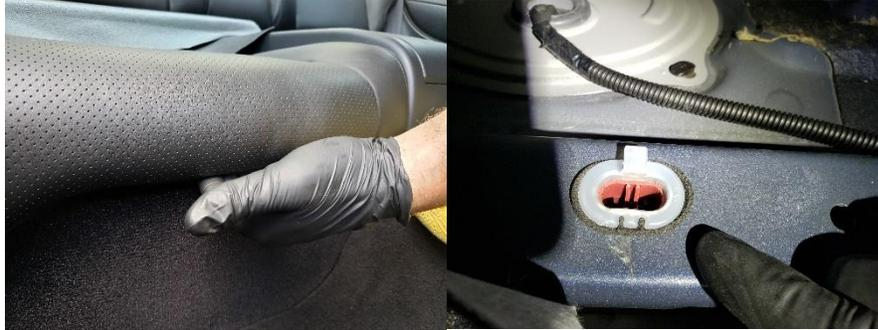
77. Once you have located the fuel pump, rotate the black tabs that hold the fuel pump cover clockwise and remove the fuel pump cover.
