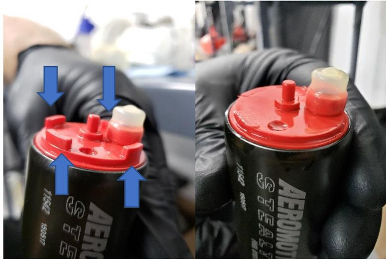
92. Install the new fuel pump sock along with the fuel pump star lock as shown below.
