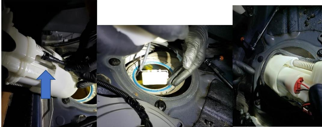
101. With the fuel pump installed into the fuel tank, make sure the orientation of the main fuel line on top of the fuel pump housing and the main fuel connector are oriented 180 degrees away from each other.
