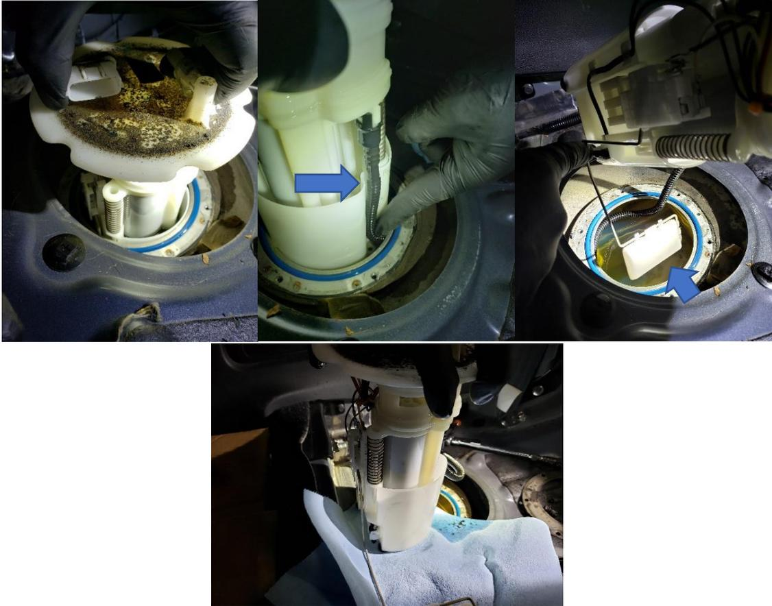
83. With the fuel pump removed out of the chassis, locate the black hose that is on the side of the fuel pump assembly. Remove this black hose by using a screwdriver to slightly press the tabs back and at the same time pulling the line off of the fuel pump assembly.
