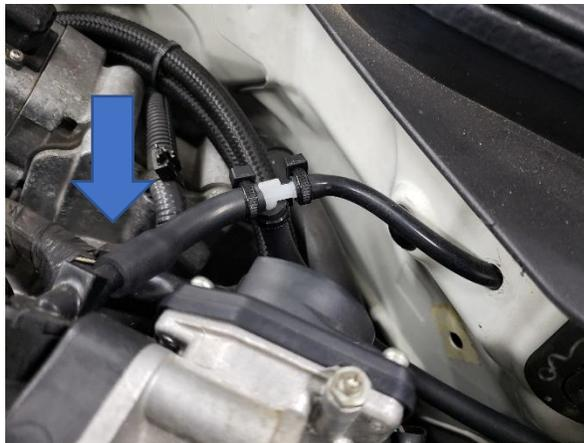
146. With the cold side piping installed, please go back at this time and install the necessary t-bolt clamps for each coupler ensuring that the pipes are tight and not loose.
