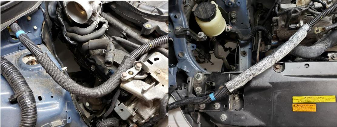
36. Locate the two sensor connectors on the lower passenger side of the engine and disconnect them at this time as seen below.
