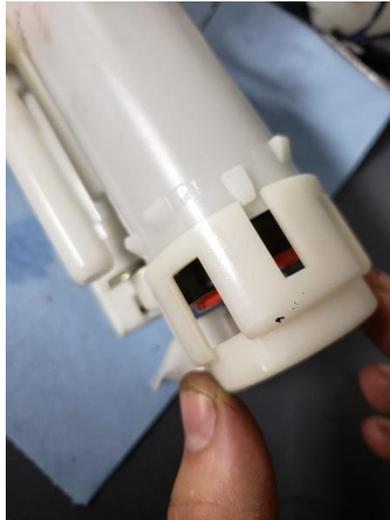
95. Since the new fuel pump does not have an OEM connector you will need to remove the current connector on the new fuel pump and on the OEM fuel pump housing. You will need to join the positive (red wire) from the fuel pump to the red wire of the OEM wiring harness and the negative (black wire) from the fuel pump to the black wire of the OEM wiring harness.
