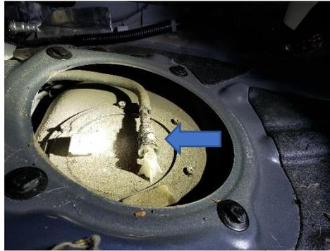
80. Pinch the clear tabs, move forward and while still holding the plastic clear tabs move the main fuel line back.
