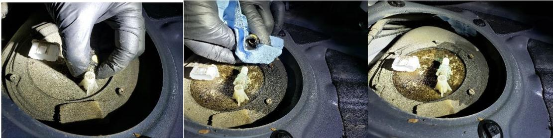
81. Locate the six 8mm bolts that hold the fuel pump bracket to the chassis and begin to remove them. Be careful to hold the fuel pump assembly down when removing the last bolt as the fuel pump assembly will want to push upwards.
