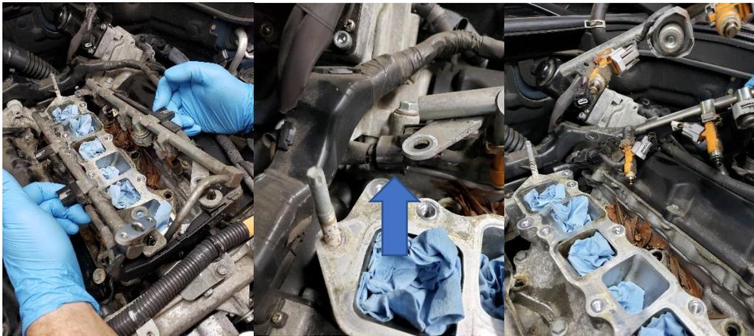
66. Once you have removed the fuel rails, please check inside the fuel injector holes on the lower intake manifold to see if any of the o rings may still be in the manifold.
