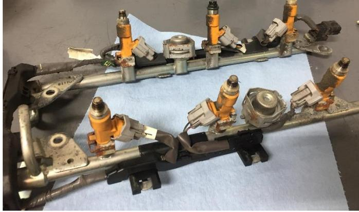
68. Remove the clip that is located on the bottom of the stock fuel injectors as seen below, gently apply pressure onto the fuel injector to remove them.
