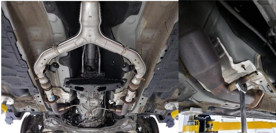
17. Remove the passenger side heat shield.
