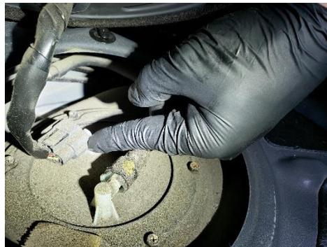
79. Once you have removed the main fuel pump connector, locate the main fuel line, and be sure to have a towel handy as you will need it to catch any residual fuel from removing the fuel line.
