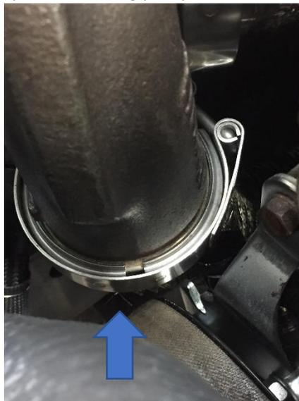
127. Install the turbo downpipe clamp onto the downpipe to secure it to the turbo as seen below.
