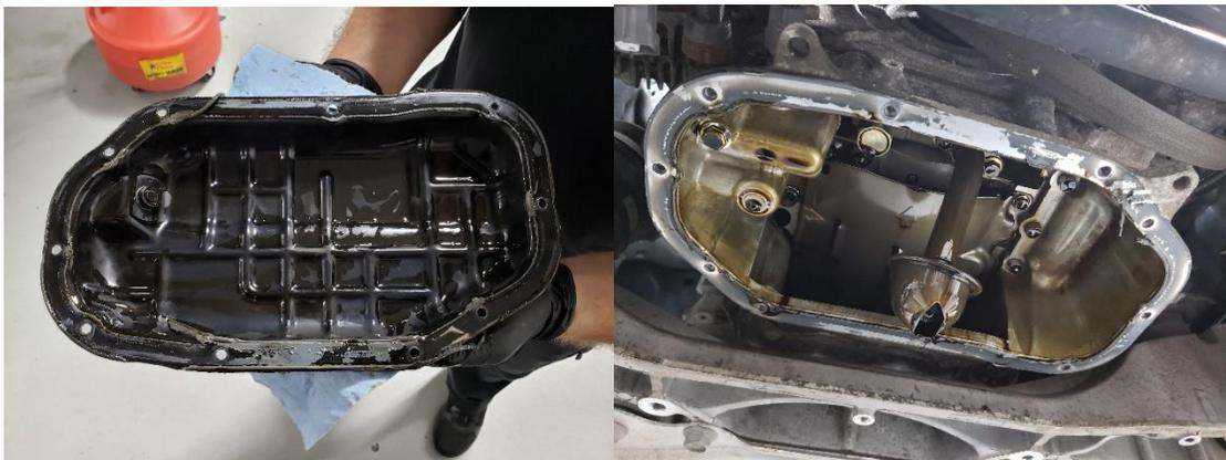
109. Remove the two (12 mm) bolts that hold the oil pick up as you will be adding a spacer to allow the pick-up tube to work properly with the new spacer.
