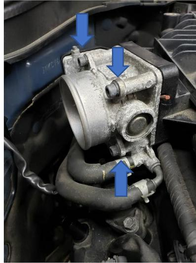
*\*Make sure to not touch the butterfly on the inside of the throttle body when removing them as damage can occur to the throttle body\**
