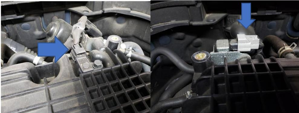
55. Remove the two bolts that hold the stock evap lines and vacuum lines as seen below on the back of the throttle bodies.
