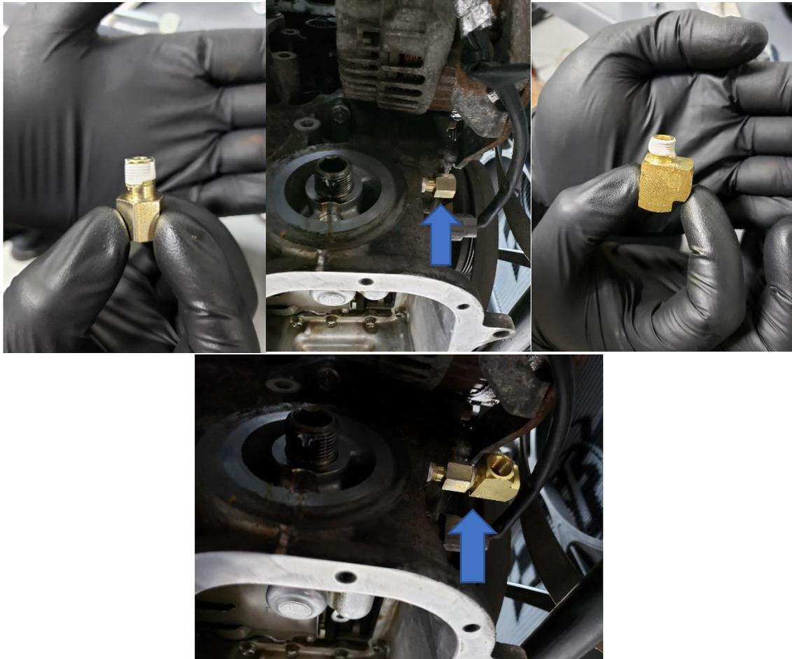
112. With both of the gold fittings installed, reinstall the OEM oil pressure sensor into the port that is closest to you and install the silver -4 oil feed fitting into the adjacent opening.
