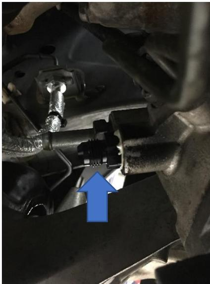
49. Route the high-pressure power steering line from the power steering rack adaptor fitting to the power steering pump adaptor fitting. When routing the line be sure to route the line above the hard line as pictured below and close to the engine as you make your way up to the power steering pump.
