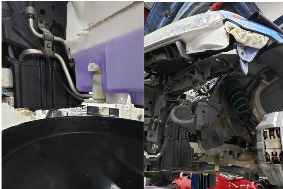
11. Once the fender liner has been removed, relocate the horn as shown below.
