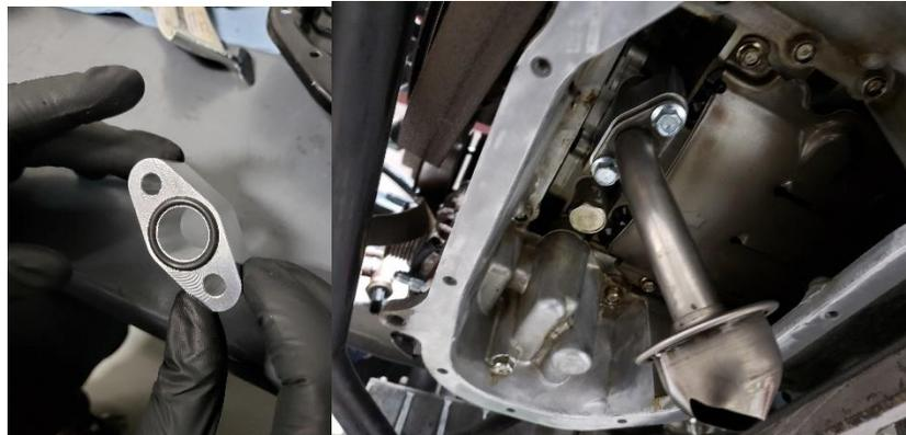
114. Using RTV, apply a film on the outer edge of the lower oil pan and install the oil pan spacer onto the lower oil pan. Repeat this process with the oil pan spacer and install it onto the vehicle as seen below.
