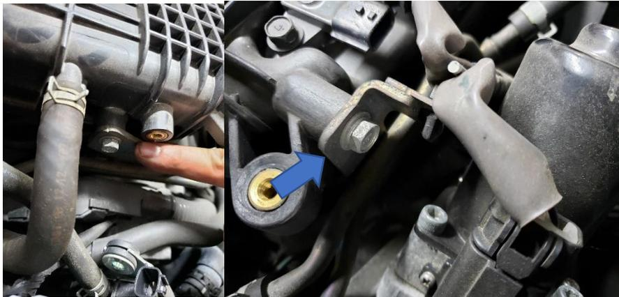
56. Disconnect the two vacuum lines to the manifold that are located on the back of the throttle bodies.
