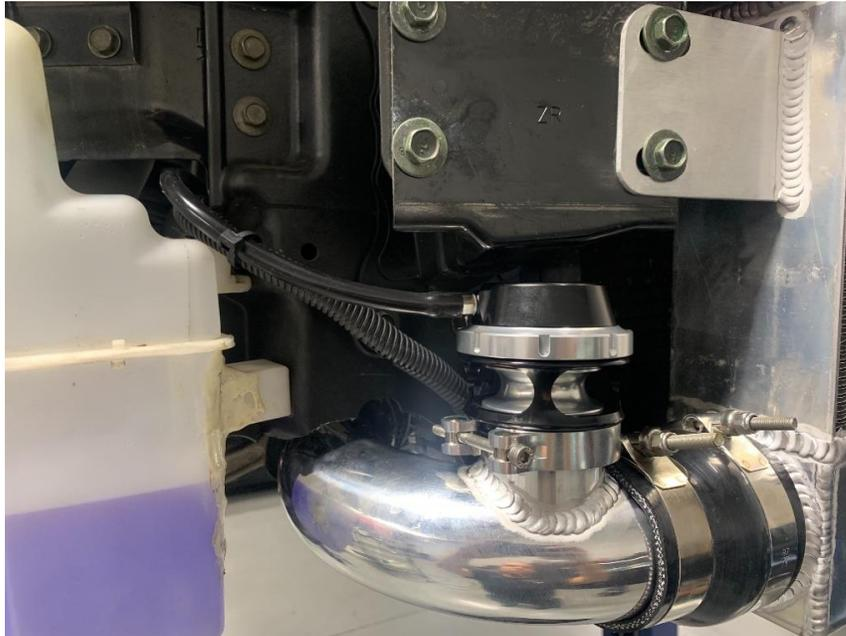
145. Once you have installed the blow off valve, install vacuum hose onto the top fittings and route the two hoses towards the intake manifold via a plastic three way tee.
