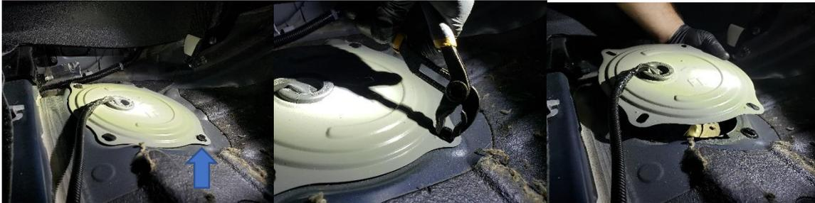
78. Pick up the fuel pump cover and locate the main fuel pump connector and remove the connector.
