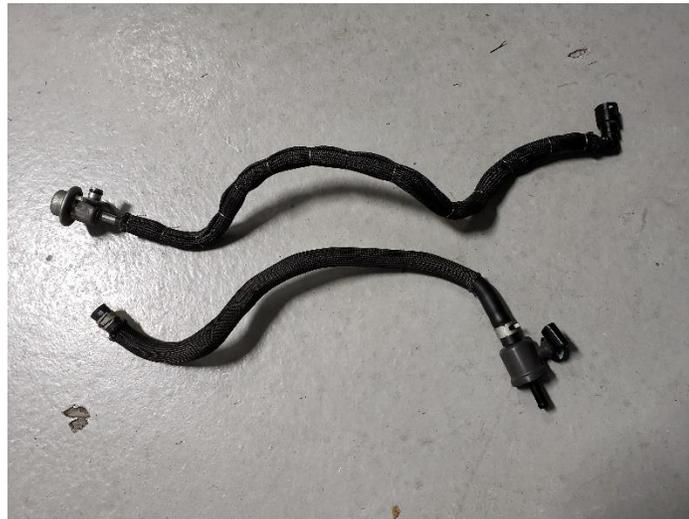
42. You will now need to move to the bottom of the vehicle near the passenger side of the transmission. The three lines that are already heat wrapped will need to be heat wrapped with another layer of heat wrap. You will need to cut out three sections of heat wrap which will include an 8", 5" and 3" section. These sections will then need to be zip tie to the harness as seen below.
