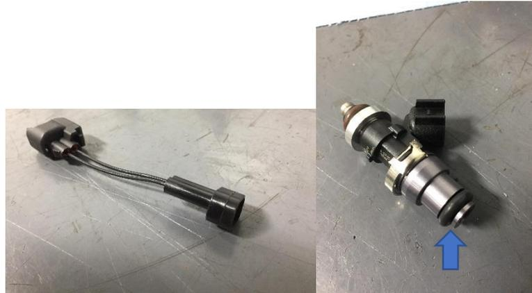
***\*Be sure to orient the connector 180 degrees away from the metal tab on the fuel rail\****
