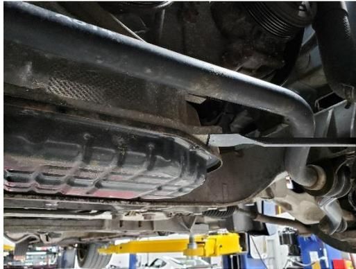
**Caution:** You will need to slowly work the screwdriver up and down to remove the oil pan spacer as the RTV that is holding the lower oil pan spacer has hardened over time.
