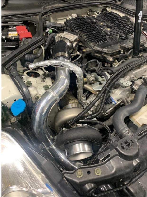
134. Zip tie both lines together up until you get to the front of the engine timing cover as seen below. Route one of the lines to the driver's side coolant hard line and secure using the hose clamps provided as seen below.
