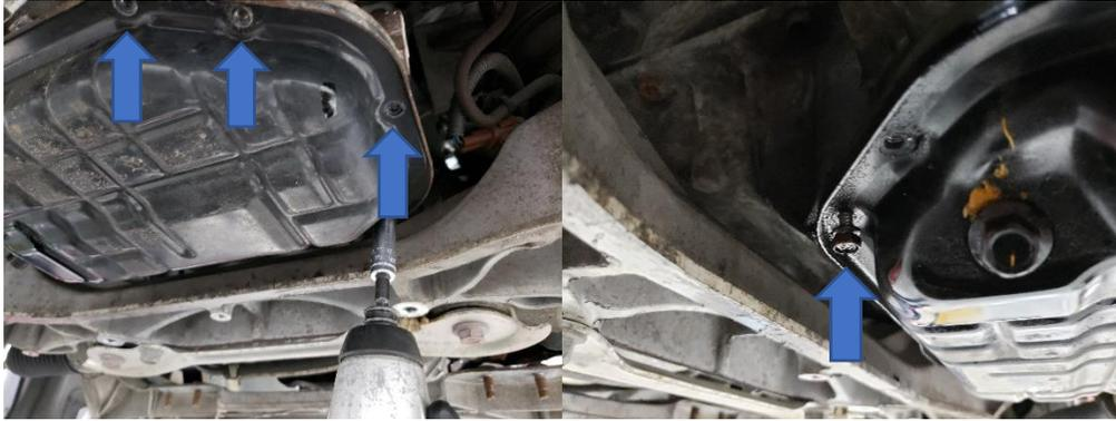
107. With the bolts removed from the lower oil pan spacer, use a flat head screwdriver and slowly begin to remove the oil pan spacer as seen below.
