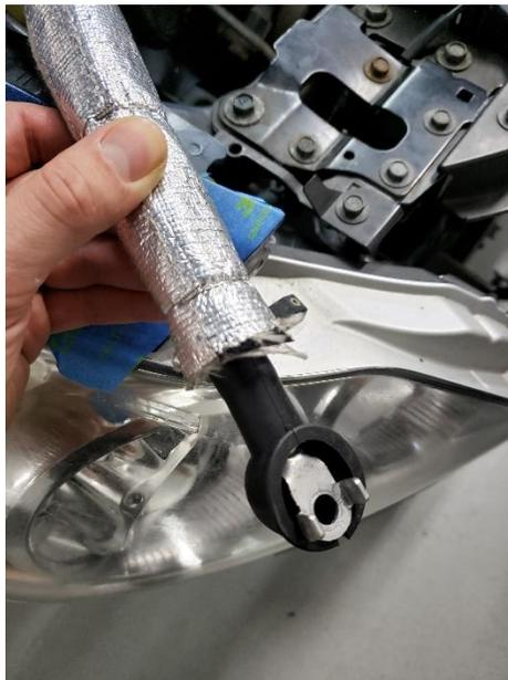
33. Remove the starter cable from the dual rubber grommet that is holding the alternator wire as pictured below.
