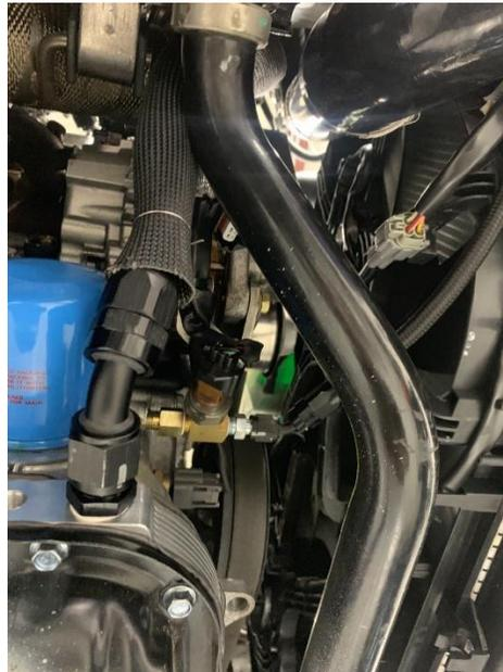
137. Install the oil drain line onto the black AN fitting on the oil pan spacer as seen below.
