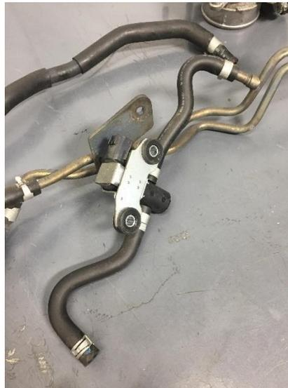
133. Install the black coolant lines that have been provided in the kit labeled HR\_SMCL1 & HR\_SMCL2. The coolant lines both have a 45 degree fitting, the longer line will need to go to the far left part of the turbo.
