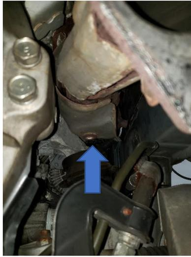
20. Remove the fuel line bracket and green clip as seen in the photo below.
