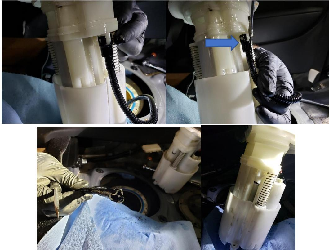
84. Remove the fuel pump assembly out of the vehicle and drain any excess fuel that may remain in the fuel pump assembly.
