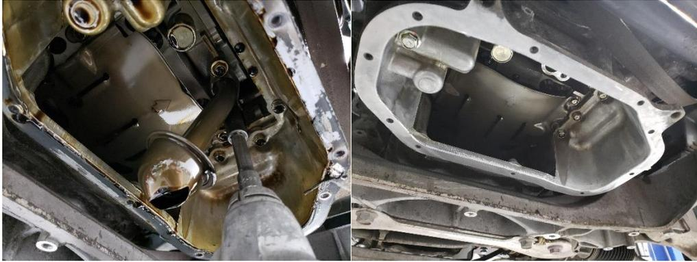
110. Locate the OEM oil pressure sensor and remove the connector to the sensor and the sensor using a **1 1/16" oil pressure socket**.
