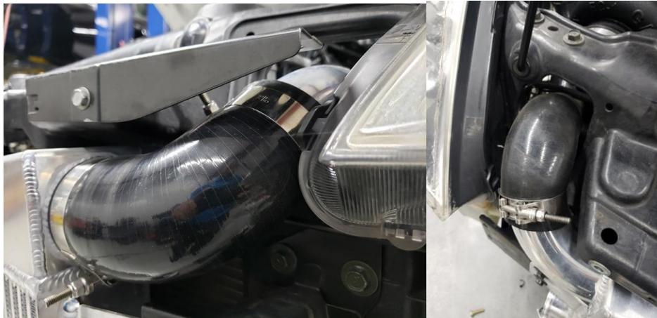
141. Install the single reducer coupler onto the bottom endcap of the intercooler and the one 45 degree 2.5" coupler onto the turbo. Once you have installed these couplers, proceed to installing the charge pipe.
