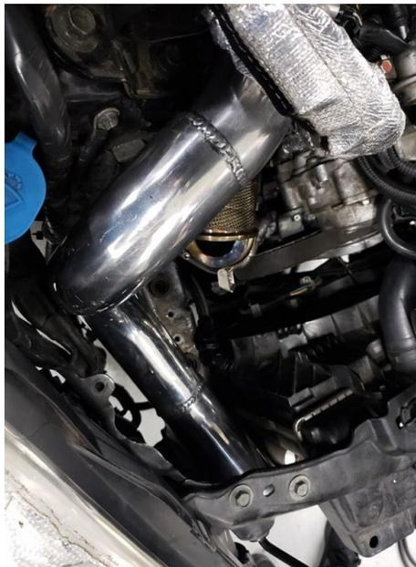
125. Prior to installing the turbo ensure that the compressor side of the turbo is clocked towards the radiator fan assembly. Also install the top portion of the downpipe as seen in the picture below.
