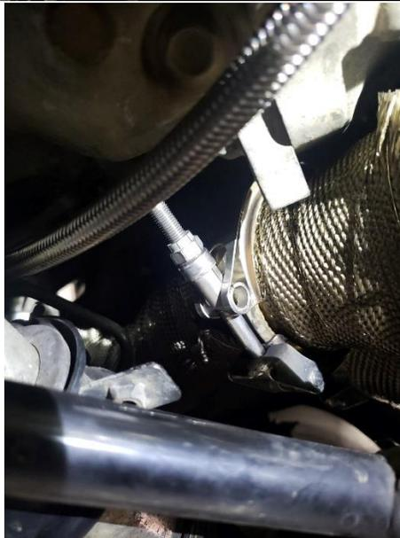
123. With the up pipe installed, you will now need to trim part of the frame to allow for the passenger side charge pipe to clear the turbo, which can be seen below.
