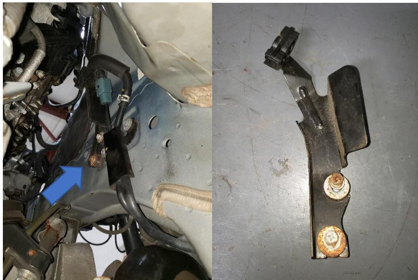
21. Proceed to unhook the fuel line via the green clip on the line, at this point, you will start to leak fuel, make sure you have a drain bucket underneath the vehicle to catch the fuel as you remove the line.
