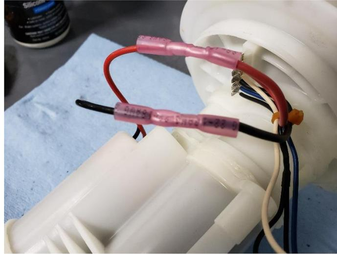
96. With the fuel pump now wired to the OEM fuel pump housing, you will need to clean any residual that may be in the fuel pump bottom housing prior to installing the fuel pump bottom housing.
