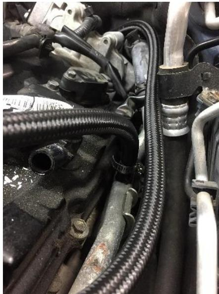
135. Route the other line with the 45 degree fitting to the rear of the engine and secure it onto the hard line as seen below.
