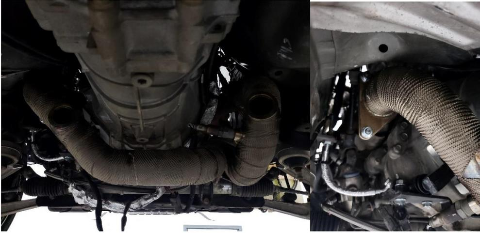
121. With the crossover section installed, install the rear O2 sensors into the proper bung location and be sure to route the wiring away from the piping.
