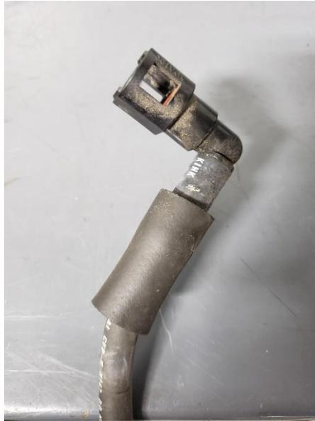
41. You will now wrap these two lines with the black heat sleeve, one will require a 21.5" section and the other will require a 16" section, which can be seen below.
