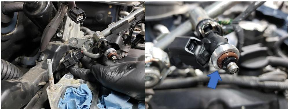
71. With the fuel injectors and fuel rail installed, proceed to installing the fuel hard line as seen below using the two 10mm and one 12mm bolt. Please lubricate the oring on the one end of the hard line and check that the o ring is not torn.
