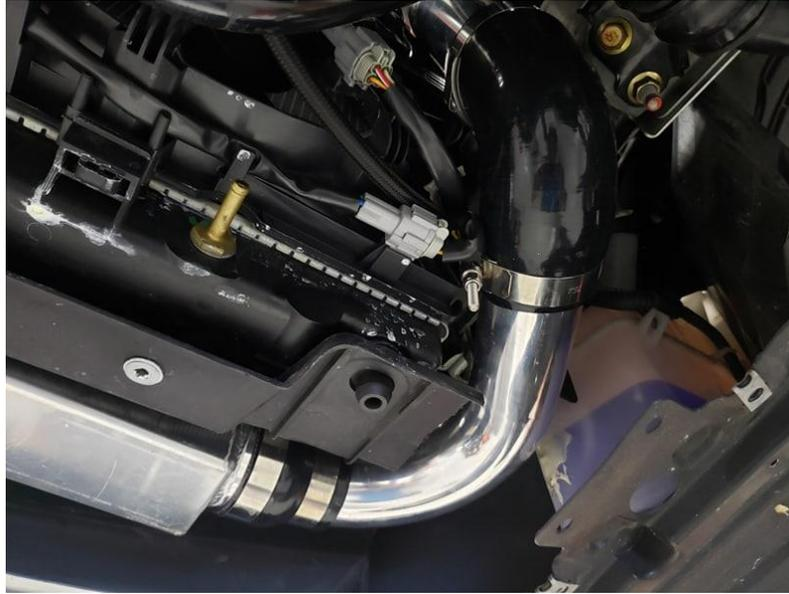
142. Install the two 2.5" to 2.75" couplers to the throttle bodies for each side.
