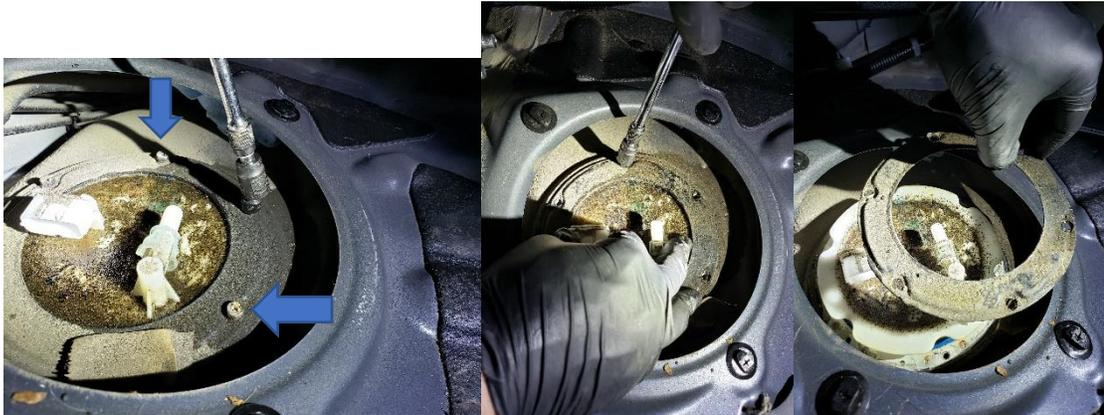
82. Begin to remove the fuel pump assembly out of the vehicle, taking caution for the black hose that can get caught on the chassis while removing the fuel pump. Slightly apply pressure to this line while removing the fuel pump assembly in a diagonal manner making sure that the fuel level sensor does not get damaged upon removal.
