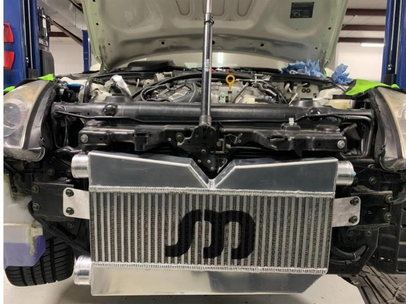
140. Install the two 90 degree couplers onto the top of the of the intercooler, installed the passenger side charge pipe and the driver side charge pipe.
