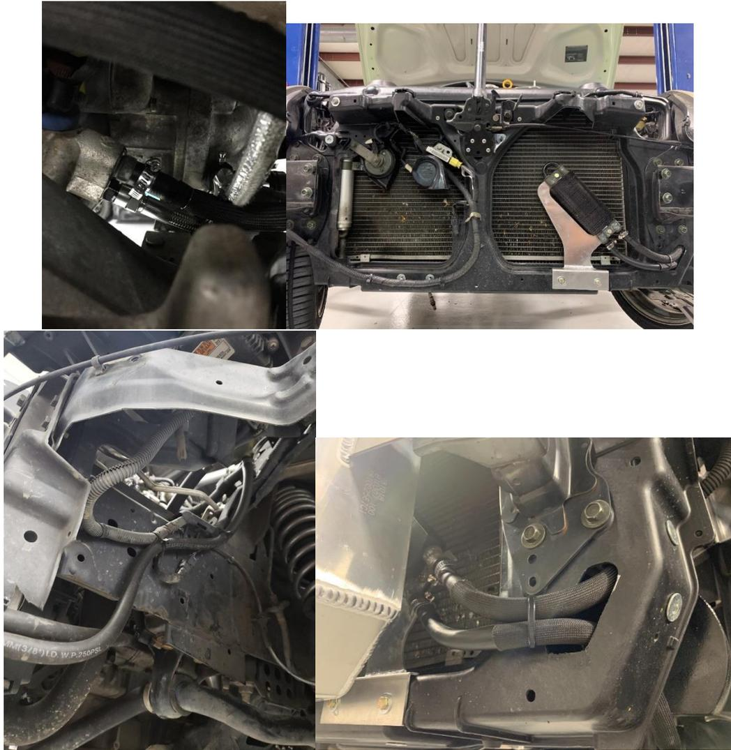
52. With the power steering lines routed, locate the rubber mount on the top of the passenger side motor mount and remove it.
