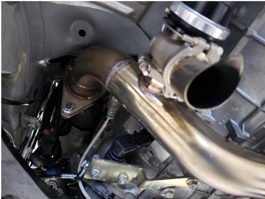
122. Install the up pipe onto the crossover section and be sure to use the 3" v-band that has been provided. Note to orient the clamp as shown in the picture below.
