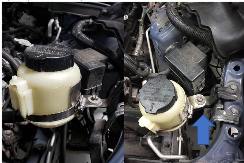
47. With the power steering pump installed and the power steering reservoir relocated, you will need to run the new power steering lines for the reservoir. The vertical fitting that comes off the power steering reservoir will need to go to the top of fitting for the power steering oil cooler. The diagonal fitting that comes off the power steering reservoir will need to go to the power steering hard line on the power steering pump.
