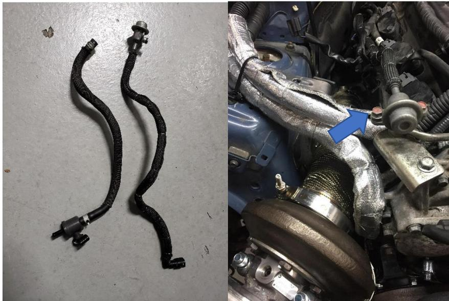
129. With the downpipe mounted to the turbo, slide the bottom portion of the downpipe into the top downpipe from the bottom of the vehicle. The tabs should line up and use the bolt provided to lock the downpipe into place. Use the rubber mount provided to secure the lower portion of the downpipe onto the cross brace once you have secured the downpipe.
