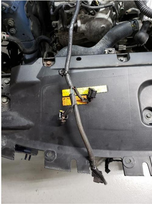
38. Install the reflective heat sleeve over the small harnesses first and then the larger portion of the same harness as seen below. Once heat wrapped, zip tie the power steering sensor connector to the larger portion of the harness as seen below. With this kit, we remove the power steering sensor.
