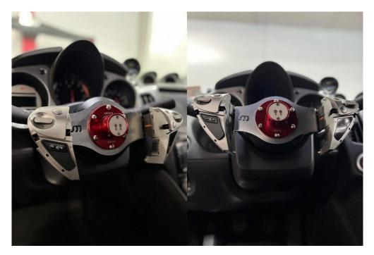
8. Install the steering wheel and ensure that nothing is touching or rubbing.
