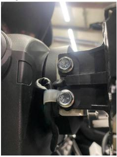
5. Be sure to run the wire through the bracket for the horn prior to installing the quick release adaptor.
