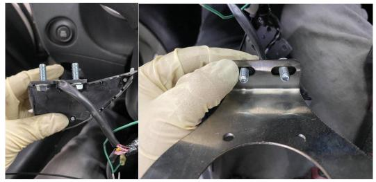
2. Install the provided nuts onto the bolts that are holding the switch to the bracket.
