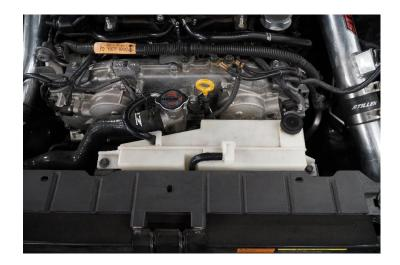
3. Begin by removing the two bolts that hold the factory coolant reservoir in place:
