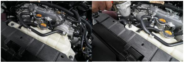
4. Remove all the coolant that is in the reservoir prior to raising the coolant reservoir out of the stock location. Once all the fluid has been removed, loosen the clamps that hold the one heater hose to the engine and the other hose that is below the coolant reservoir.
