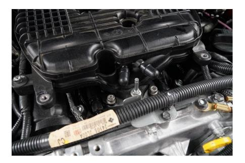
12. Install both fittings from the previous step onto the proper line for each side. The longer line will go on the passenger side and the shorter line will go on the driver's side:
