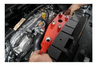
8. Remove the coolant hose that was on the original coolant reservoir and trim as shown in the picture (white line where screwdriver is pointed to). You may need to trim an additional inch once it has been test fitted to ensure a nice smooth transition of the hose:
