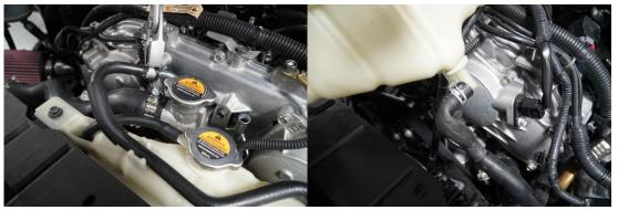
5. Remove the stock PCV hoses and PCV valves from the driver and passenger side and install the aftermarket PCV delete fittings that have been provided in the kit:
