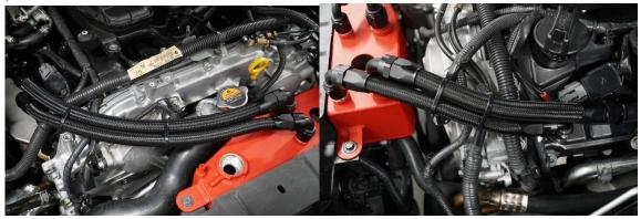
15. If your vehicle is a 2015+ you will need to block the factory expansion tank hose off using the provided billet plug. Simply shorten the hose, push the plug in, and reinstall the OEM spring clamp.
