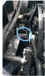
7. Install the bottom coolant hoses onto the SOHO coolant catch can and then install the catch can combo into the original location. Install the 137kPa radiator cap at this time.
