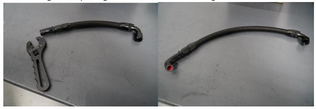
13. Begin by installing the PCV line on the driver's side first and then the breather line and repeat the same procedure on the passenger side:
